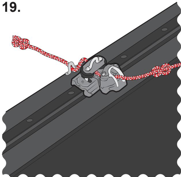
Pass the traveller line through the cleat on the traveller car and through the eyelet on the beam.
