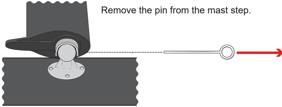
Remove the pin from the mast step.
