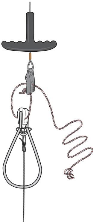
Connect trapeze wires to elastic.
