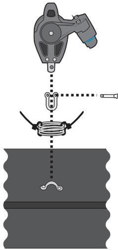
Add jib blocks to front beam. This will be easier if you use cable ties to compress the spring then cut zip ties once jib blocks are shackled on.
