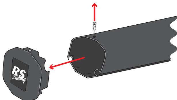
Using a screwdriver, remove all 4 screws.
