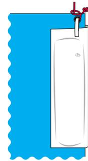
5. Gently feed the mainsail and the mast-head float into the mast track.
