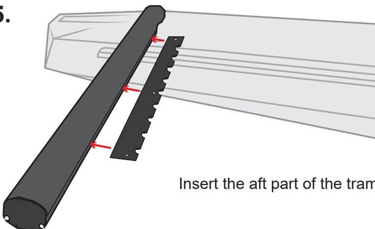
Insert the aft part of the tramp into the track on the stern beam.
