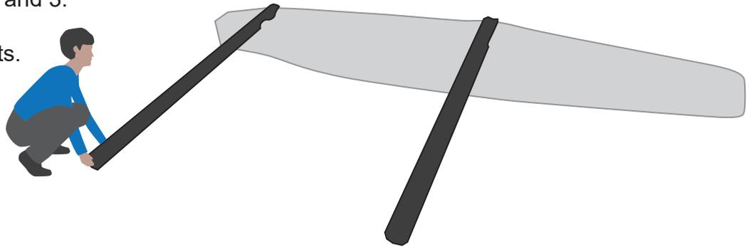
9. Push the 6mm x 1860mm batten through the reinforcement pocket in the front edge of the tramp.
