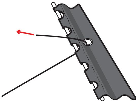
Pass the elastic back to the transom and through the cringle at the back of the tramp.
