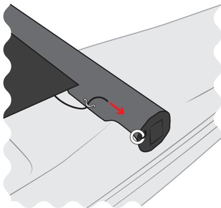
Pass the elastic back under the tramp to the opposite side of the boat and up through the eyelet on the aft face of the beam (mirroring the process from the other side of the boat).
