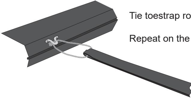
Tie toe strap ropes through toe straps and knot through eyelet.
