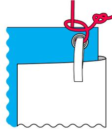
4. Fold the mast-head float loosely around the luff of the mainsail.
