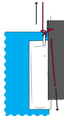
7. When the mainsail is at the top of the mast, cleat the main halyard, coil the excess halyard, and stow it in the halyard bag.
