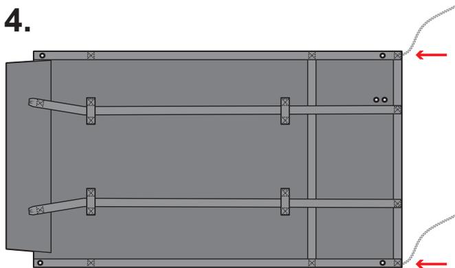
Using longest 6mm batten, poke tramp ties down seam pockets on both sides.
