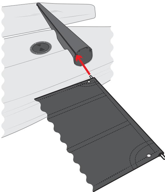
Slide the front edge of the tramp (with the batten inserted) into the track on the front beam.
