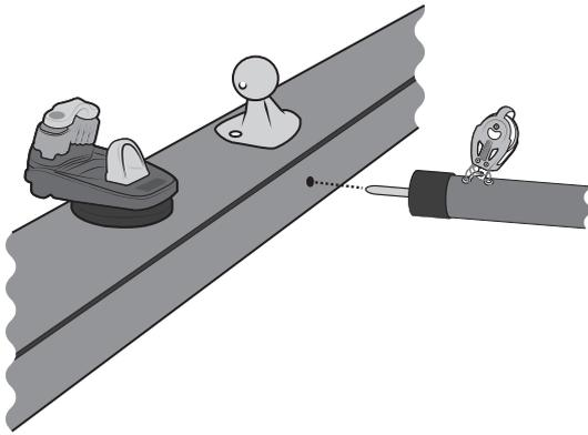
Remove the plastic cap from front beam.
