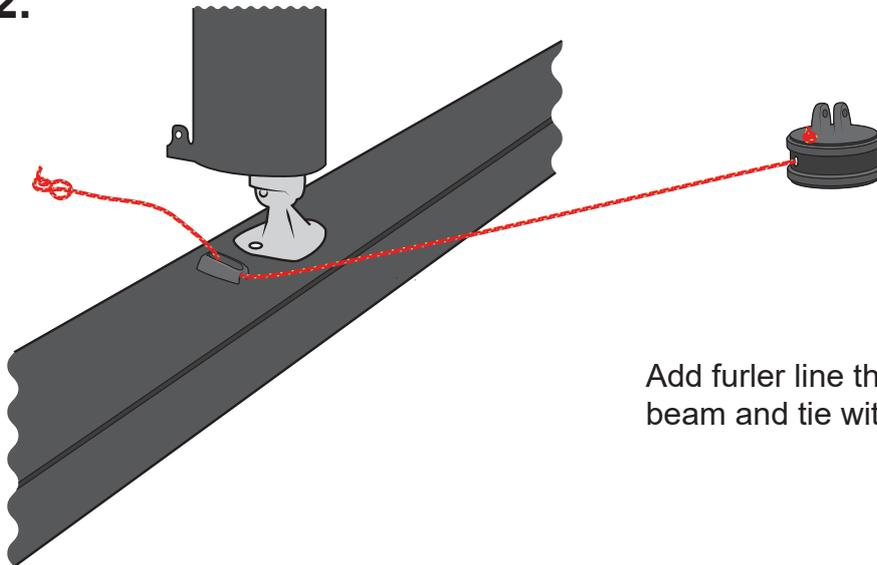
Add furler line through cleat on front beam and tie with **knot #3**.
