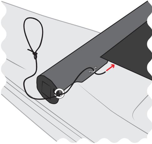
Feed the end down through the eyelet on the aft face of the beam and down under the tramp.
