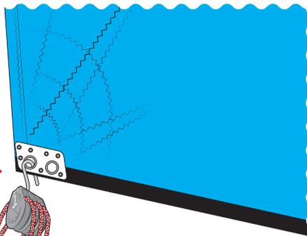
The bottom block shackles onto the traveller.
