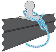
Tie the righting line around the mast step with **knot #2**.
