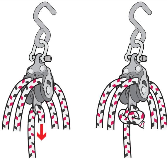
Pass the tail back up to the top block and tie onto the becket with **knot #1**.
