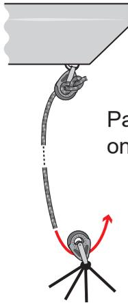
Pass the end of the mainsheet down and through the block on the mainsheet bridle.
